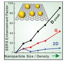
A systematic investigation of surfaceenhanced Raman scattering (SERS) in graphene-nanoparticle-hybrids is obtained by a versatile electrochemical procedure. The evolution of Raman enhancement is followed by varying nanoparticle size and density at the same location. The magnitude of SERS enhancement is found to be dependent on the vibrational mode of graphene with both electromagnetic and chemical contributions.
