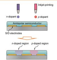
Local molecular doping via inkjet printing of dopants on a pre-coated ambipolar semiconductors is demonstrated to unipolarize and optimize complementary transistors. The mobility and turn-on voltages both for electrons and holes are precisely modulated by doping. Finally, high performance complementary ambipolar inverters are achieved by the selective inkjet printing of n- and p-type dopant.
