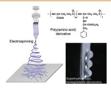
Superhydrophobic, biodegradable nonwovens are fabricated by electrospinning from a naturally occurring poly(amino acid). The nonwovens exhibit a petal-type superhydrophobicity and water droplet sticks to the surface even after it is turned over. The material design and processing is applicable to different biopolymers, and such functional materials can be useful for biomedical and environmental applications.
