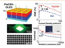
A new organic LED structure is proposed and experimentally demonstrated using a novel plasmonic nanocavity, termed "plasmonic cavity with subwavelength hole-array" (PlaCSH), to significantly enhance over conventional LEDs: i) 1.57fold higher external quantum efficiency and light extraction efficiency (55% and 60%); ii) 2.5-fold higher ambient light absorption over 400 nm band; iii) a contrast of fivefold higher; and others.
